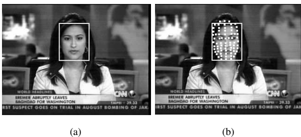
Figure 2. (a) Rectangular bounding box for the face region and (b) feature vector extraction.
